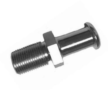
Designed as a companion part for use with single rotor latches that requires a 10mm (.394") diameter striker pin and compliance to FMVSS 206 (ECE R11).
